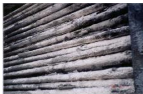
Scale at Tube Condenser
