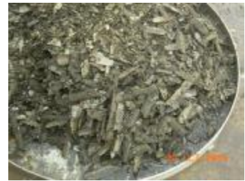
Collecting Scale from Evaporative Condenser
