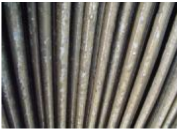
Scale at bottom of Tube
