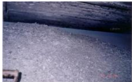
Scale came off from tube 800-900 kgs.
